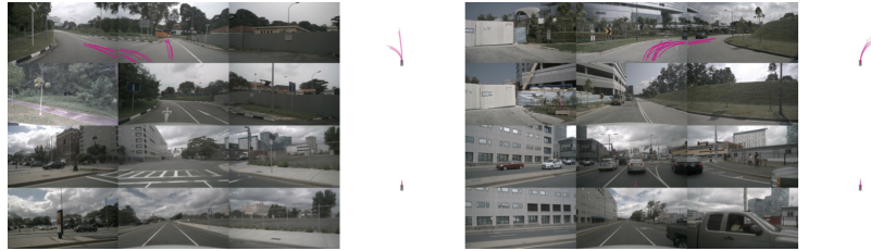
Fig. 11: We display the top 10 ranked trajectories out of the 1k templates. Video sequences are provided on our project page. Our model predicts bimodal distributions and curves from observations from a single timestamp. Our model does not have access to the speed of the car so it is compelling that the model predicts low-speed trajectories near crosswalks and brake lights.
