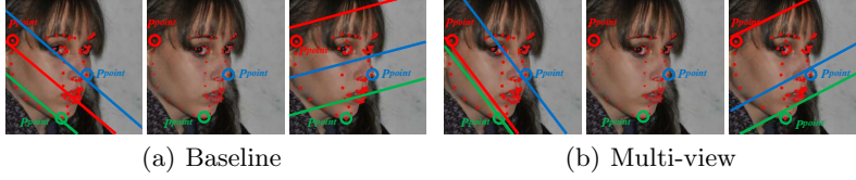
Fig. 4. Epipolar error from target to source views, (a) is the epipolar visualization from baseline network trained by 2D feature loss; and (b) is epipolar visualization of the MGCNet. The red, green and blue point means left ear bound, lower jaw and nose tip landmarks. The epipolar error of baseline is significantly larger than MGCNet.
