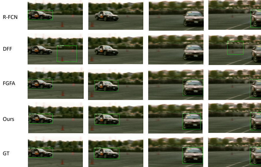
Fig. 1. Visualization comparisons between our method and R-FCN image detector, DFF video object detector.
