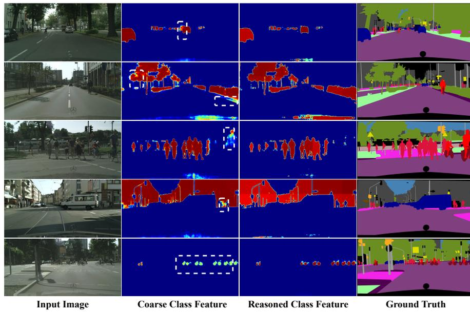
**Fig. 3.** Visualizations of class-wise features before and after graph convolution on Cityscapes validation set. From left to right: input image, class-wise feature before CDGC module, class-wise feature after CDGC module, ground truth. From top to bottom, the visualized category is car, vegetation, person, building and bicycle.
