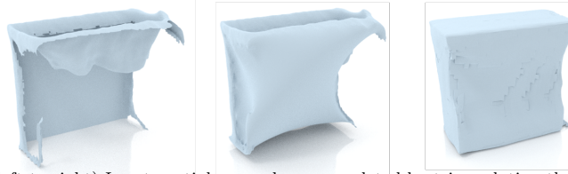
Fig. 8: (From left to right) Input partial scan, shape completed by triangulating the hole boundary and shape annotated using our tool. The hole-filling method is incapable of completing large unseen surface (the back of the bin). We use the CGAL [7] implementation for hole filling with triangulation.
