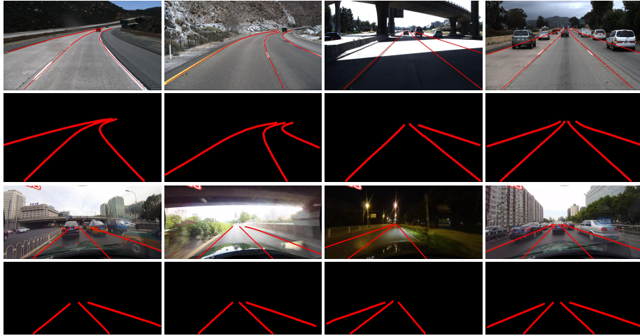
Fig. 1. More visualization results. Row 1 and 3: images with ground truth on TuSimple and CULane datasets respectively. Row 2 and 4: the corresponding visualization results of our PRNet.
