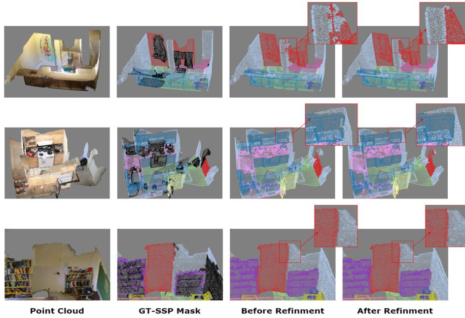
Fig. 3: Some visualization comparison examples for semantic segmentation before and after joint refinement (best viewed in color).
