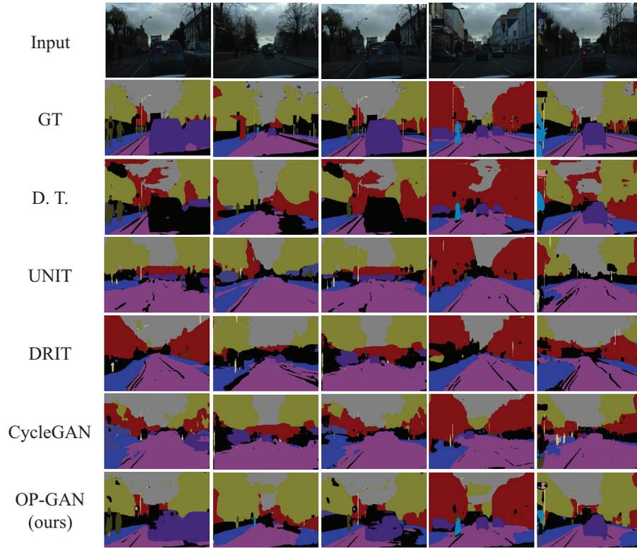
**Fig. 6.** Semantic segmentation results produced by the sunny-image-trained PSPNet for the original CamVid cloudy images and the ones translated by UNIT [22], DRIT [18], CycleGAN [37], and our OP-GAN. D. T. refers to direct transfer.
