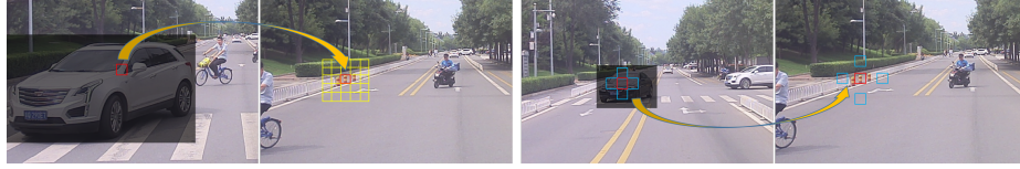
Fig. 5. Left image pair: potential color choices for a target pixel. a pixel within inpainting region find its candidate pixel (red box) from a source image. A small window of pixels around this candidate (yellow boxes) are all potential colors to fill the target pixel. Right image pair: the 4 neighbors of a target pixel are not necessarily neighbors in the source image due to perspective change. In order to get neighbor colors, we need to warp neighbor pixels into the source image by their depth value.
