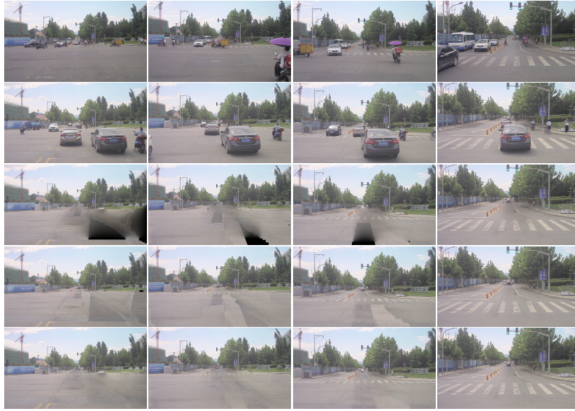
Fig. 9. 1st row: frames from video 1; 2nd row: frames from video 2 captured on a different day; 3rd row: results after Poisson color blending using video 2 only; 4th row: direct inpainting results by fusing both videos; 5th row: results after Poisson color blending using both videos.
