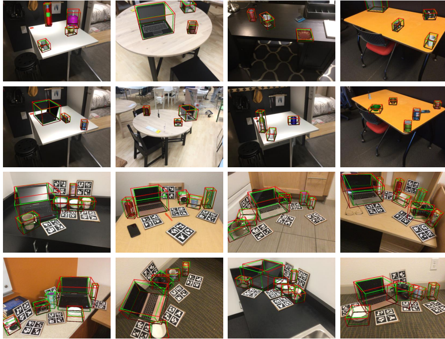
Fig. 1. We show some qualitative results of our approach (red) and their ground truths (green) on CAMERA25 (top two rows) and REAL275 (bottom two rows).
