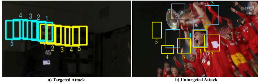
Fig. 1. Two examples of adversarial attacks for VOT. To better show the attacking results, we plot the bounding boxes in the initial frame. The numbers represent the results in the corresponding video frames. The blue box represents the predicted bounding box, and the yellow box represents the ground truth.
