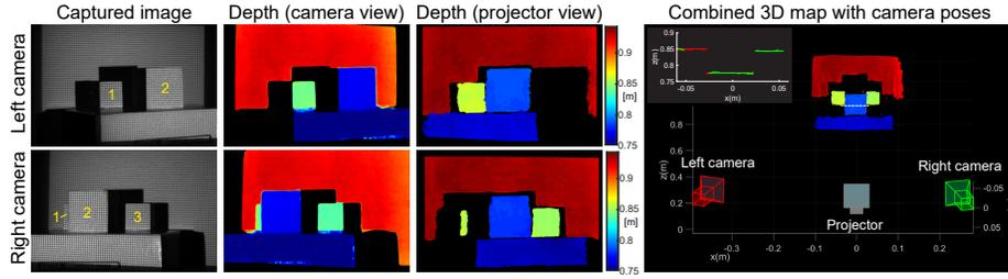
**Fig. 6.** 3D reconstruction from two cameras. Each camera only sees a part of the scene. Since our system estimates the 3D map in world coordinates, those two point clouds can be combined seamlessly. The height along the dashed scanline is plotted.
