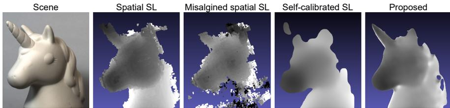
**Fig. 5.** Experimental depthmap comparisons with single-shot structured light methods.
