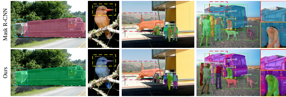
Fig. 1. Baseline Mask R-CNN (top) vs. Ours (bottom) with ResNet-101-FPN. Our approach is more adaptive for scales of objects and more sensitive on their boundaries (best viewed in color)
