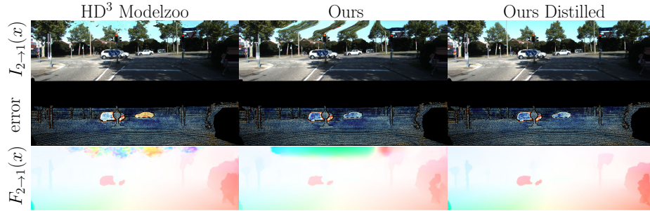
Fig. 7: Qualitative evaluation on KITTI, comparing the HD 3 modelzoo (left), our version with all contributions except distillation (center), and with distillation (right).
