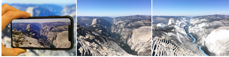
Fig. 9. An iPhone application (in the left) is used to capture the photograph (in the middle) for which precise camera pose is estimated using our method. The estimated camera pose (in the right) is used to augment the query photograph with contour lines (white) and rivers (blue).
