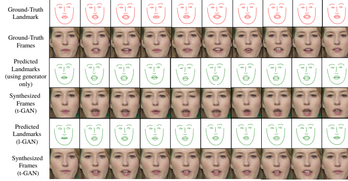
Fig. 4: Performance comparison of l-GAN using only generator (third row) and the complete GAN (fifth row). The regression-based approach cannot capture the finer details like "a" and "o" of lip motion without the help of the discriminator.
