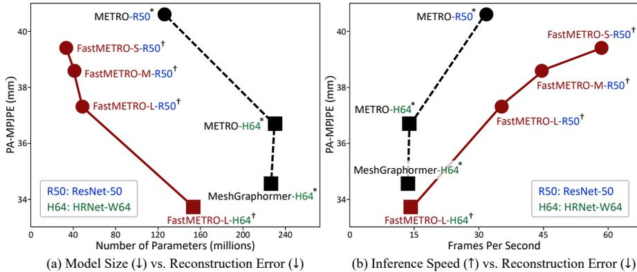
**Fig. 1.** Comparison with encoder-based transformers [24, 25] and our models on Human3.6M [14]. Our FastMETRO substantially improves the Pareto-front of accuracy and efficiency. † indicates training for 60 epochs, and \* denotes training for 200 epochs.
