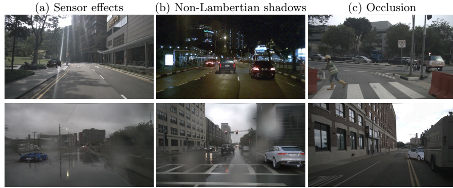
Fig. P: Qualitative results – failure cases. (a) The virtually inserted object may not pass exactly the same environment and signal processing pipeline as the real-world captured scene pixels, e.g. the virtual object cannot reconstruct the halo effects of the sun and blurry regions caused by rain drops on the camera. (b) We assume a Lambertian scene surface when rendering the shadows, and thus the quality of editing results may decrease for wet specular road surfaces on rainy days. (c) Our occlusion handling relies on depth ordering, and may generate artifacts when the scene depth map prediction is inaccurate.
