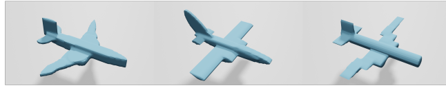
Fig. A. Reconstruction results by setting constraints on the extrusion plane orientation. Left: Top Extrude. Middle: Side Extrude. Right: Front Extrude.
