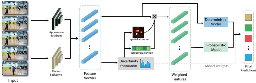
Figure 2: **Overall framework.** Firstly, feature vectors are constructed by concatenating the appearance features and motion features. Then we estimate the uncertainty based on the input and use the quantified uncertainty to generate the spatial-temporal attention. Finally, the prediction is made by dynamically combining both the deterministic model and probabilistic model, whose inputs are original features and attention-weighted features respectively.
