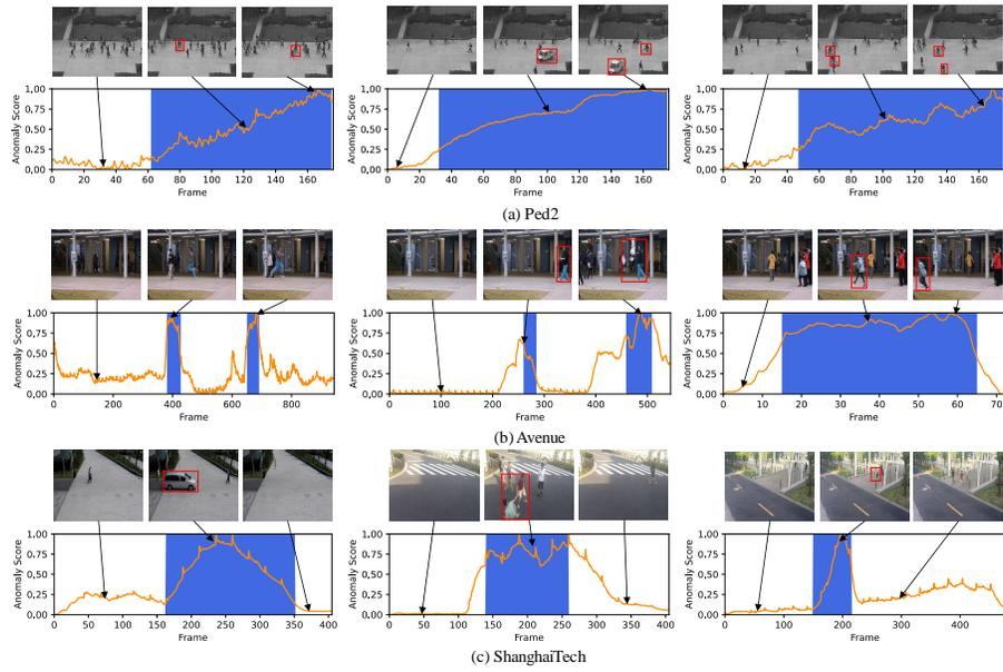
**Fig. 2.** Anomaly score curves of several test video clips of our method on Ped2, Avenue, and ShanghaiTech datasets. Royalblue regions represent ground truth anomalous frames. It shows that the anomaly scores rise dramatically when anomalies occur and decrease when anomalies disappear. (Best viewed in color.)
