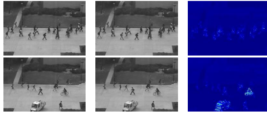
Fig. 2. Example of frame prediction on Ped2 dataset. The first row is a prediction example of normal event, and the second row is a prediction example of an abnormal event. Left column: the real frame. Mid column: the prediction frame. Right column: the prediction error map. (Best viewed in color.)
