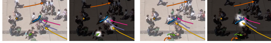
Fig. 4. Attention maps at the 1st (left) and 20th (right) frames in UCY students003 . Trajectories of the pedestrian under prediction appear in blue. The other colored lines with arrows are the observed neighbors. Yellow dots denote stationary neighbors.
