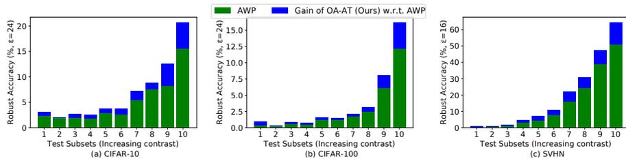
Fig. 5. **Evaluation across test subsets of increasing contrast levels:** Here we plot the gain in robust accuracy of the proposed defense OA-AT over AWP [30]. The proposed defense achieves higher gains as contrast increases, verifying that the proposed approach is more robust to the Oracle-Invariant white-box attacks on High-Contrast images.
