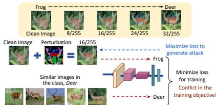
Fig. 2. **Issues with Standard Adversarial Training at Large- $\epsilon$ :** An adversarial example generated from the original image of a frog looks partially like a deer at an  $\ell_\infty$  bound of  $16/255$ , but is trained to predict the true label, Frog. This induces a conflicting objective, leading to a large drop in clean accuracy.
