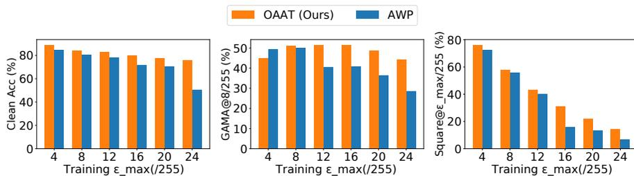
Fig. 6. **Results across variation in training  $\epsilon_{max}$ :** While the proposed approach works best at moderate- $\epsilon$  bounds such as 16/255 on CIFAR-10, we observe that it outperforms the baseline for various  $\epsilon_{max}$  values  $\geq 8/255$  as well.
