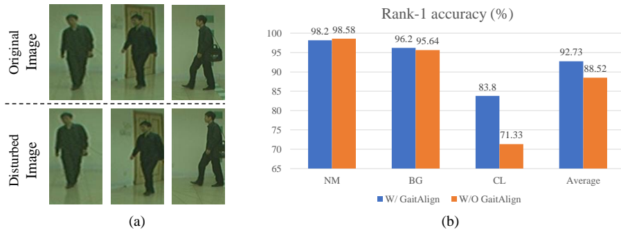
Fig. 6. (a) The original images (top) vs. the disturbed images (bottom). We make random pixel offset to the disturbed images, including vertical and horizontal direction. (b) The ablation study for the GaitAlign module. The results are reported on CASIA-B* after disturbance
