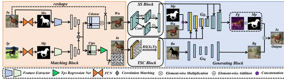
**Fig. 2. The Overview of the UFO-PT architecture.** For simplicity, we take “horse” as an example for input. Given the unpaired images  $I_a$  and  $I_p$  providing appearance and pose information, the matching block first aligns them and establishes the two types of warpings. Then, the generating block yield the transformed output  $I_o$  based on the different injected warped intermediates from SS block and TSC block, respectively.
