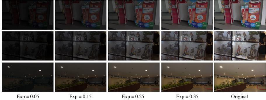
Fig. 5: The proposed EC-Zero-DCE is able to generate low-light images with different exposure levels, while keeping the intensities of saturated pixels unchanged.
