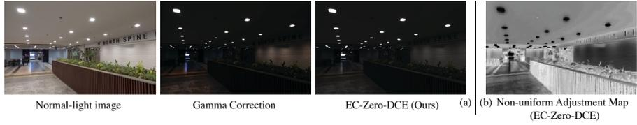
Fig. 4: (a) Comparisons between the proposed EC-Zero-DCE and Gamma correction for generating low-light images. (b) The non-uniform adjustment map suggests that EC-Zero-DCE performs spatially-varying luminance adjustment.
