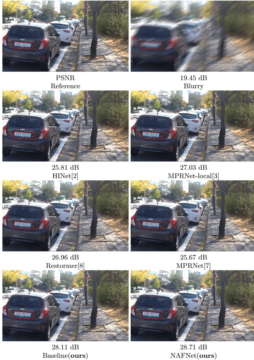
Fig. 2: Additional qualitative comparison of image deblurring methods
