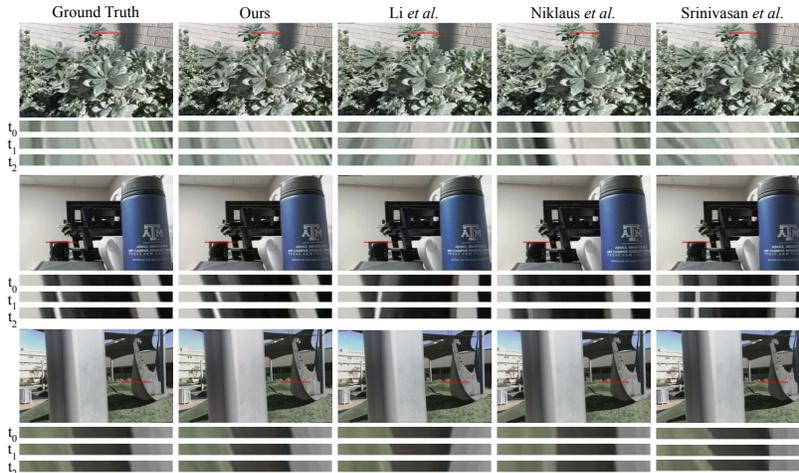
**Fig. 6.** We qualitatively compare our reconstruction with ground truth and other state-of-the-art techniques. We show the top-left view of  $t_0$  and EPI images from three consecutive LF frames ( $t_0, t_1, t_2$ ). As can be clearly seen from the EPI images, our technique consistently provides accurate reconstructions.
