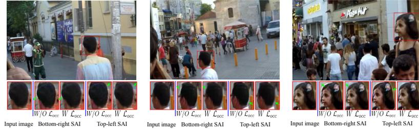
**Fig. 7.** The model trained without disocclusion handling leads to a halo-like artifact around depth-edges in the SAIs of the frames. With the proposed disocclusion handling technique, the network learns to accurately fill-in the disoccluded pixels.
