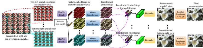
**Fig. 5.** A supervised residual refinement block is used to further improve the reconstruction quality of the LFs. The transformer block attends to the spatio-angular information in the estimated LF and the input frame  $I_t$  to predict the refined output.
