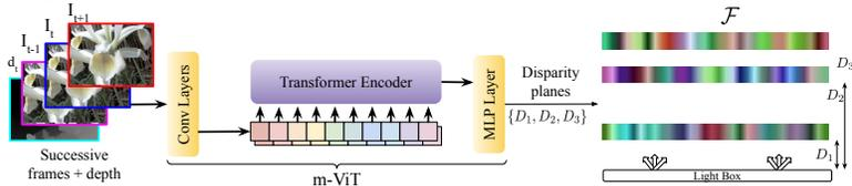
**Fig. 3.** We use an m-ViT block [3] to predict the displacement between the different layers of the TD based low-rank representation. Each of the layers in  $\mathcal{F}$  approximately represent a scene depth plane. Instead of keeping the layers static/fixed, a scene-specific displacement value will move the layer to a depth plane where it can best represent the scene.
