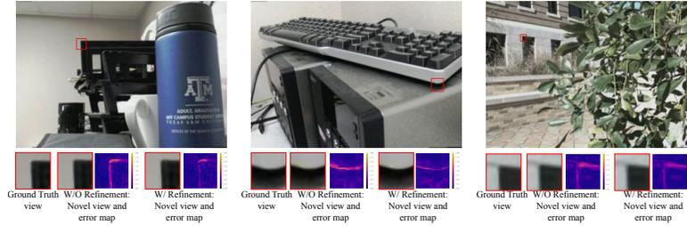
**Fig. 9.** The error map between the reconstructed and ground-truth shows that supervised refinement improves reconstruction at depth-edges. The refinement module corrects the baseline discrepancy. The refinement block utilizes the spatial information in other SAIs through angular attention and optimizes the positioning of depth-edges correcting the baseline discrepancy between synthesized and ground truth LF.
