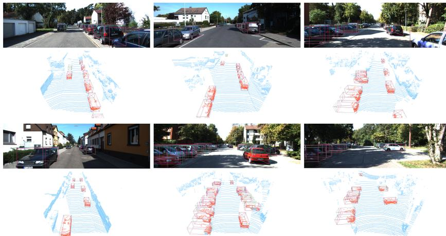
**Fig. 2.** Qualitative results of Graph-Po on the KITTI *val* set. We show detection results in six scenes, where the upper is the scene image, and the lower is the front view detection results.
