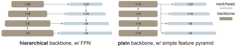
Figure 1: A typical hierarchical-backbone detector (left) vs. our plain-backbone detector (right). Traditional hierarchical backbones can be naturally adapted for multi-scale detection, e.g. , using FPN. Instead, we explore building a simple pyramid from only the last, large-stride (16) feature map of a plain backbone.
