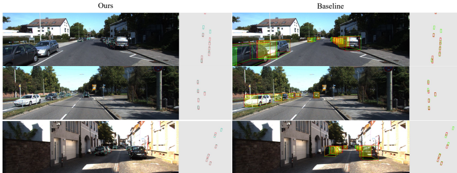
Fig. 3. The qualitative results on the KITTI val set. Rather than representing an object as a bounding box, we utilize semantic keypoints to represent an object. The red boxes represent the ground truth, while the green boxes represent the prediction.
