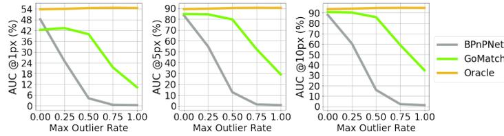
**Fig. 4.** Influence of keypoint outlier rate. In contrast to prior work BPnNet [10], GoMatch is significantly more robust against keypoint outliers thanks to the more powerful attention-based architecture as well as our novel formulation of matching bearing vectors instead of cross-modal features.
