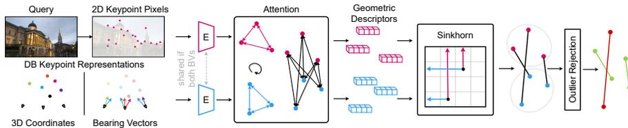
**Fig. 3.** GoMatch components overview. The query image and database keypoints first undergo a feature encoder  $E$  to generate per-point features. We share encoders in the query and database branch when database points are represented as bearing vectors otherwise not. These features are refined in the attention layer and then used in the Sinkhorn matching stage to establish an initial set of candidate matches, from which erroneous matches are filtered with an outlier rejection layer.
