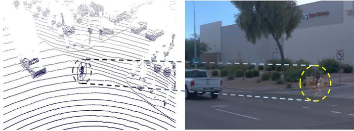
**Fig. 3.** Examples of multi-modalities copy paste data augmentation. The left one is the visualization of LiDAR point. The right one is the visualization of camera images. The cyclist in the yellow is pasted on by eq.5 and eq.6.
