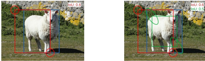
(a) Assigning predictions to ground truth is non-trivial in probabilistic OD. The prediction can either be considered a true positive with bad uncertainty estimates or a false positive. (b) mAP and [13] prefer the red prediction with larger IoU. Our method considers uncertainties and multiple assignments, and finds the green prediction a more probable match to the blue ground truth.
