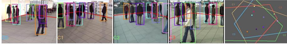
**Fig. 4.** The detection results at frame 3225 of the EPFL Terrace dataset: from left to right, camera views C0, C1, C2, C3 and the top view. Each detected pedestrian is represented by a distinguished colour consistent across different views. The red rectangle on the ground is the AOI. The field of view of each camera is shown in the top view.
