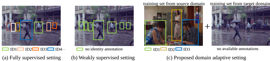
Fig. 1: Comparison of three person search settings. (a) Fully supervised setting: bounding boxes and identity annotations are available. (b) Weakly supervised setting: only bounding boxes annotations are available. (c) Domain adaptive setting: neither bounding boxes nor identity annotations on the target domain is accessible, and there exists obvious domain gaps between different domains, e.g. , the size of human crops. The network is trained with both the labeled source domain and the unlabeled target domain images.
