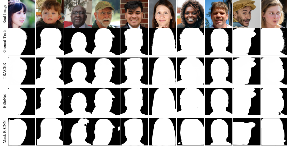
Fig. S1: Qualitative comparison of masks. We manually annotated ground truth masks (second row). TRACER produces masks very similar to the ground truth. BiSeNet also shows acceptable performance, but it often misclassifies the background as a foreground (3rd, 9th column) and vice versa (10th column). Mask R-CNN is relatively poor in quality, especially near the borders of the mask.
