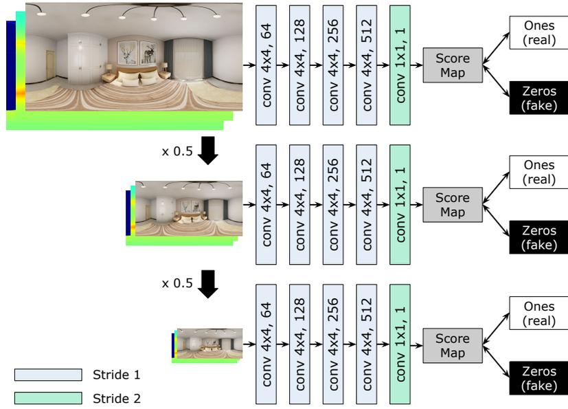
**Fig. 3.** The proposed discriminator network architecture.
