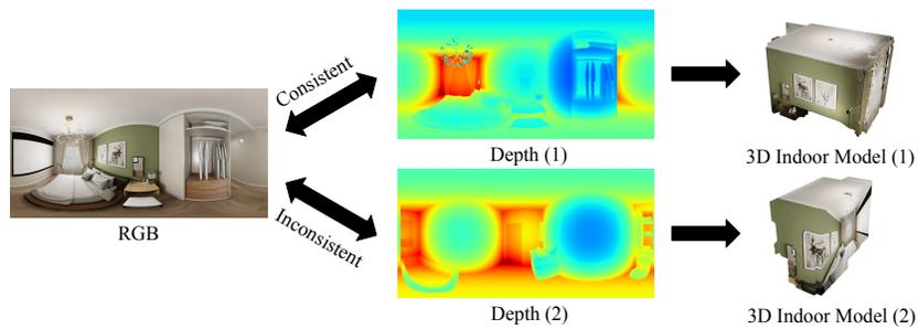
**Fig. 4.** Visual results of the semantic inconsistency. Depth (1) is well-aligned with RGB. Depth (2) is misaligned with RGB.
