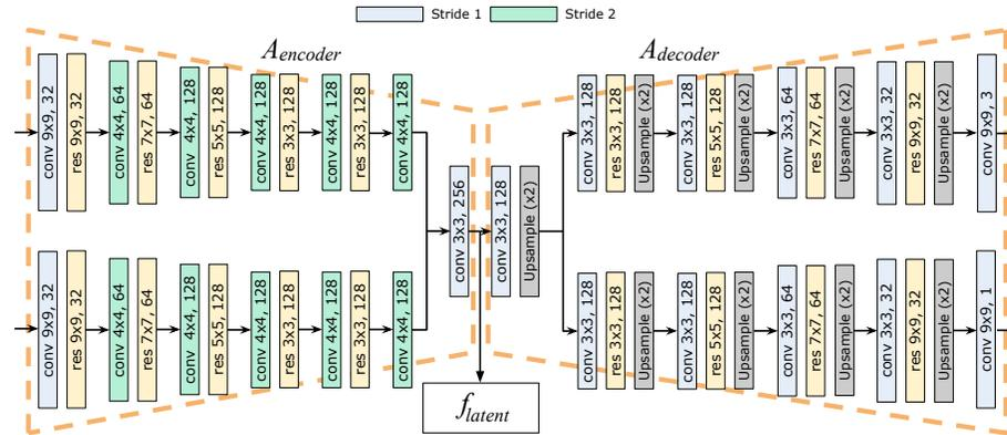
Fig. 2. The proposed auto-encoder network architecture.
