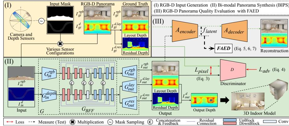
**Fig. 3.** Overall structure of our bi-modal indoor panorama synthesis (BIPS) framework. Our framework takes RGB-D input provided by various sensor configurations, integrates the bi-modal input data with BFF branch in the generator network, and jointly trains to synthesize layout depth and residual depth. Then, the perceptual quality of the synthesized RGB-D panorama is measured by proposed FAED metric.
