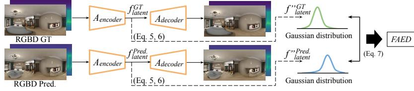
**Fig. 4.** The proposed FAED metric for RGB-D panorama quality evaluation. It measures the distance of the distributions of latent features extracted from the pre-trained auto-encoder network on RGB-D panorama.
