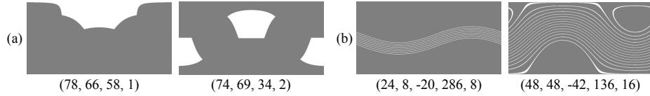
**Fig. 2.** Sampled input masks. (a) Input mask of cameras and perspective depth sensors with parameters  $(\delta_H, \delta_V, \psi, n)$  and (b) mechanical LiDARs with  $(\delta_L, \delta_U, \psi, \omega, \eta)$ .
