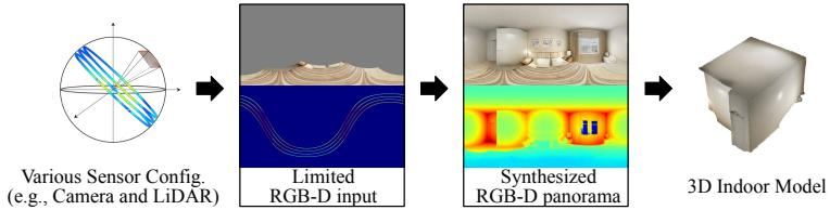
**Fig. 1.** Overall scheme for our BIPS framework, which takes RGB-D input from cameras and depth sensors in various configurations and synthesizes an RGB-D panorama.
