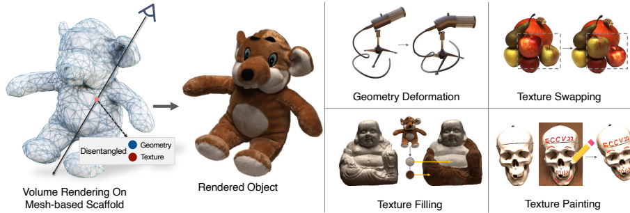
Fig. 1. NeuMesh. We present a novel representation for volumetric neural rendering, which encodes the neural implicit field with disentangled geometry and texture features on a mesh scaffold. With the locally separated latent codes, our representation enables a series of editing functionalities, including mesh-guided geometry deformation, designatable texture swapping, filling and painting.
