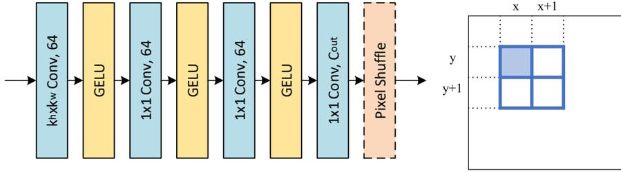
**Fig. 1.** Detailed architecture of the mapping module. Only **Fig. 2.** The receptive field of the last mapping module of each branch contains the pixel field of  $r = 4$  for the pixel shuffle layer. colored in blue.
