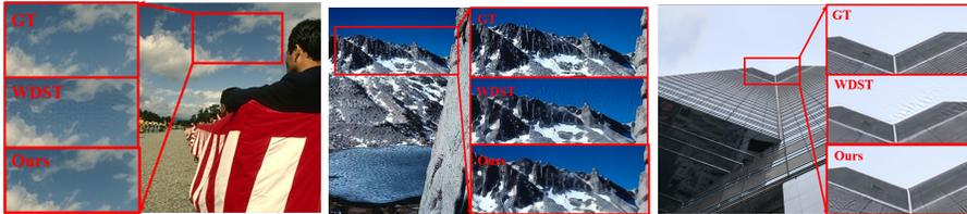
Fig. 9: Comparison between our method and WDST [1]. WDST generates non-existent textures in low-frequency regions, which do not occur in our results.
