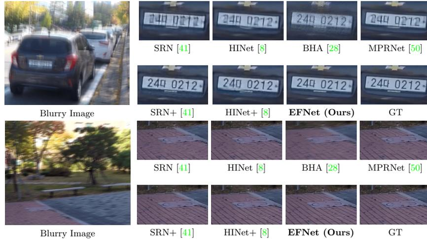
Fig. 4: **Visual comparison on GoPro.** SRN+ and HINet+: event-enhanced versions of SRN and HINet using SCER. Compared to image- and event-based state-of-the-art methods, our method restores fine texture and structures better.
