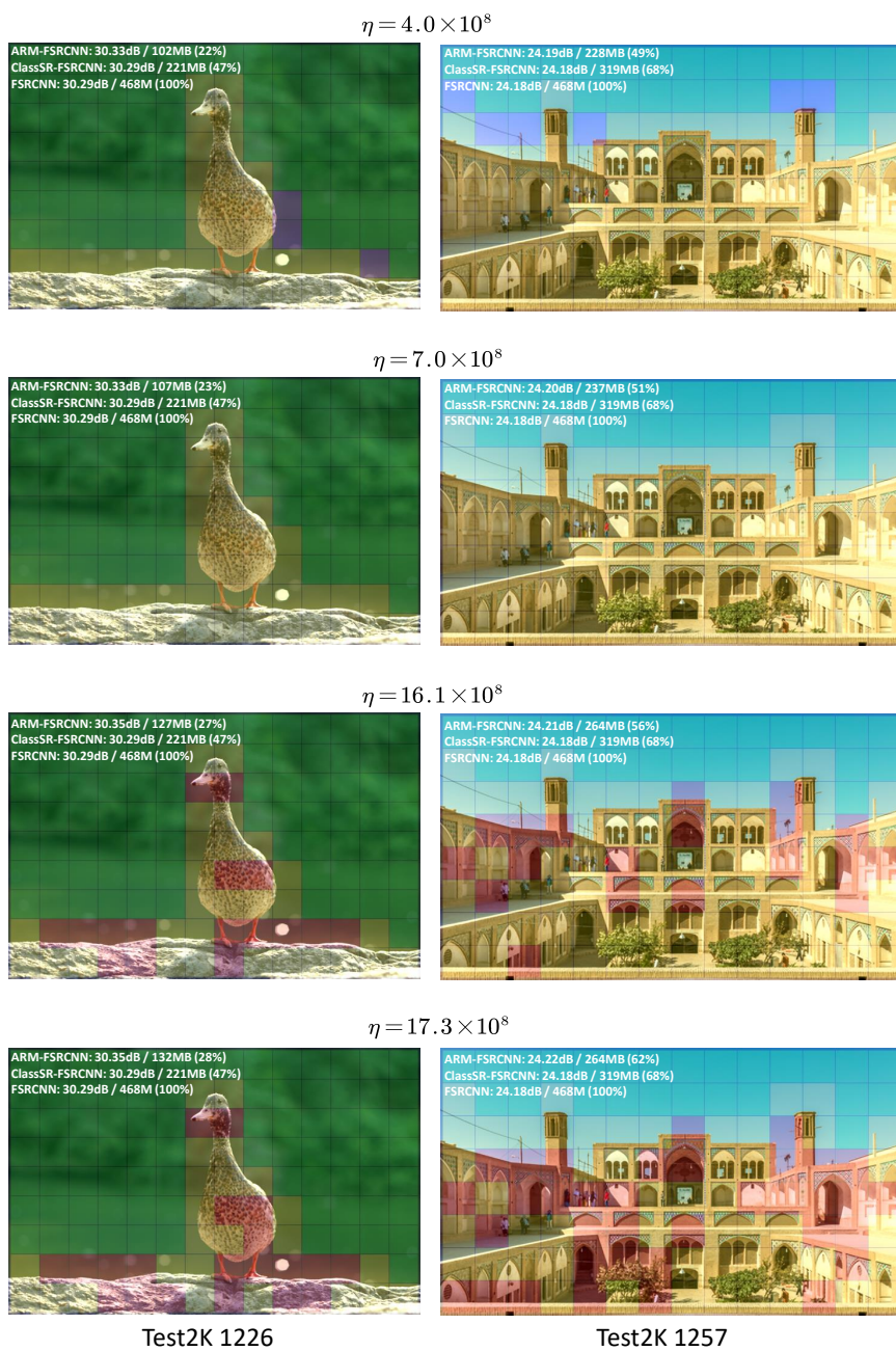
Fig. 3. Examples of super-resolution visualization of ARM-FSRCNN with different \eta . The green, blue, yellow and red masks on the patch indicate that ARM uses interpolation, subnet_1 , subnet_2 and subnet_3 for super-resolution of the patch, respectively.
