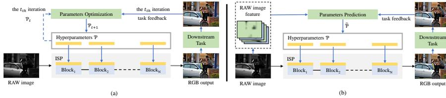
**Fig. 1.** Illustrations of different ISP tuning methods. (a) Previous methods leverage a mapping between the parameter space and high-level evaluation metrics based on differentiable approximations or hardware ISP. (b) Our proposed framework firstly constructs an attention-aware prediction network between RAW sensor data and parameter space, and then follows the previous work to create the mapping function between the parameter space and high-level evaluation metrics.
