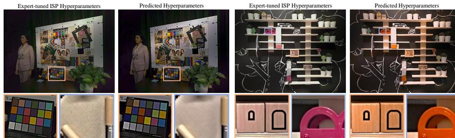
**Fig. 4.** Comparison of Expert-tuned hyperparameters and our method. These images are processed by a synthetic ISP described in Sec. 3 to match the image quality of the reference images generated by the Qualcomm Spectra580 ISP.
