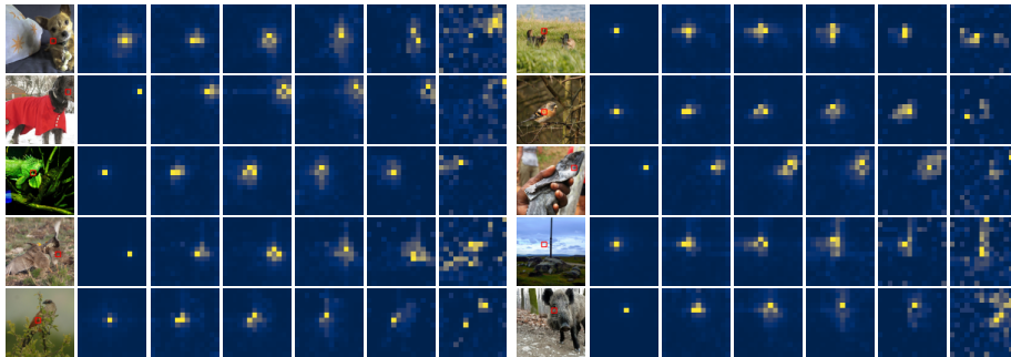
Fig. 3: Our method can generate data-dependent attention weights without token-token interactions. The attention weights in shallow layers usually focus on local regions while the weights of deeper layers adaptively attends to the shape of the whole object.
