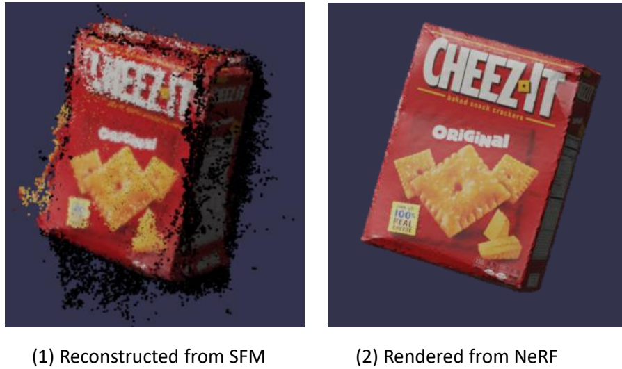
Fig. 4: Quality of images rendered using 3D model generated using a standard structure-from-motion pipeline. In comparison, NeRF can generate high-quality images without needing high-quality 3D models.
