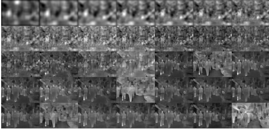
Figure S2: Feature maps upsampled by CARAFE with increased training iterations. From left to right, from top to bottom, CARAFE starts from the interior and then spreads outside.
