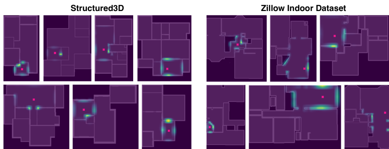
Fig. 5. Investigation into floor plan saliency for inferring layout at a given location from a global floor plan. The query location is marked with a pink cross, and computed saliency is overlaid onto the floor plan. The floor plan comprehension module demonstrably learns to differentiate between visible and invisible structure for the query locations when computing their descriptor.
